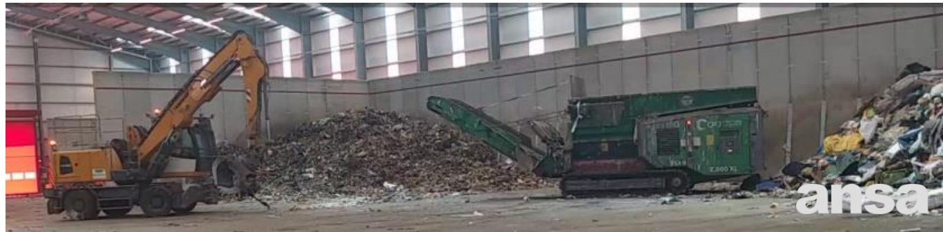
Image: Residual waste being shredded at the Environmental Hub ready for onward transfer to third party energy from waste providers
